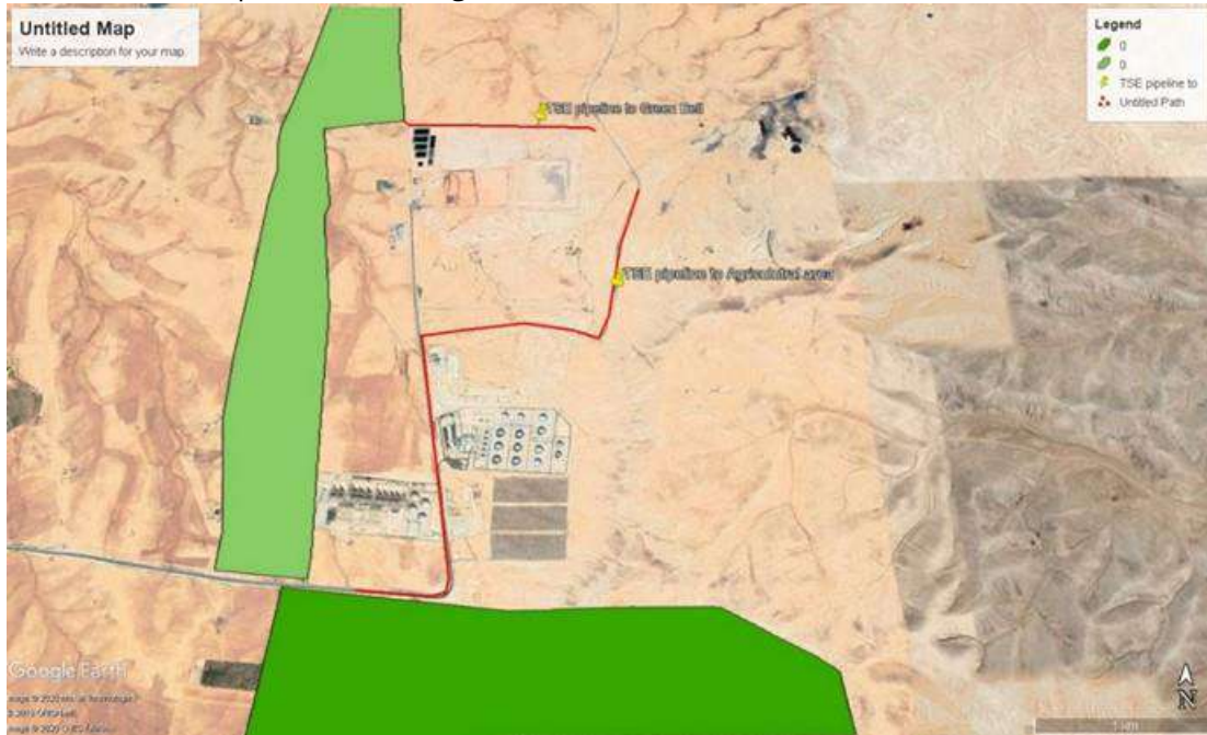
Figure 3.1. Pipeline paths (in red color) for the transfer of treated effluent to the green belt and agricultural investment areas
